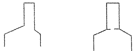
Central Tip : 1ml ,2ml ,3ml ,5ml ,10ml Eccentric Tip: 10ml , 20ml , 30ml ,50ml
